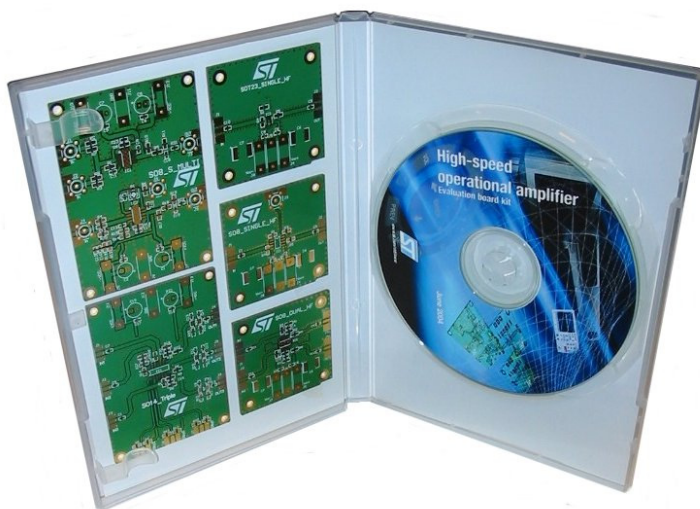
Figure 25: Evaluation kit for high-speed op-amps
